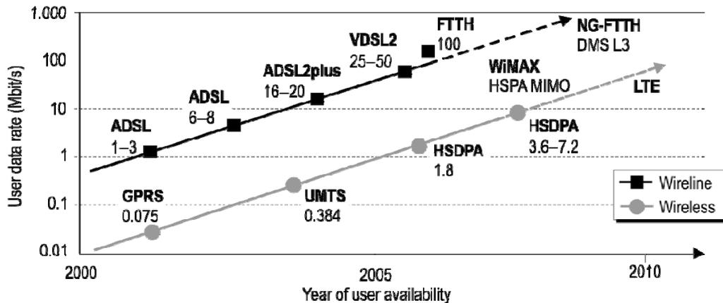
Figure 8: Development of wireline and wireless data rates in access technologies<sup>86</sup>
