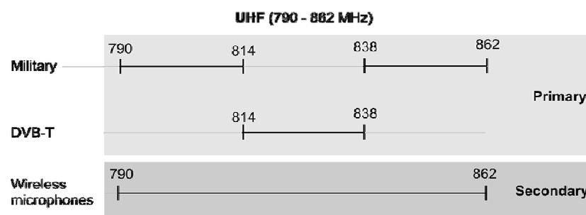
Figure 5: Spectrum utilization in Digital Dividend Frequencies<sup>63</sup>
