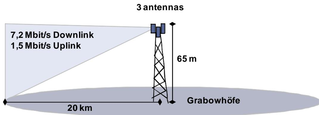
**Figure 9: Wireless Broadband Pilot Setup in Grabowhöfe**
