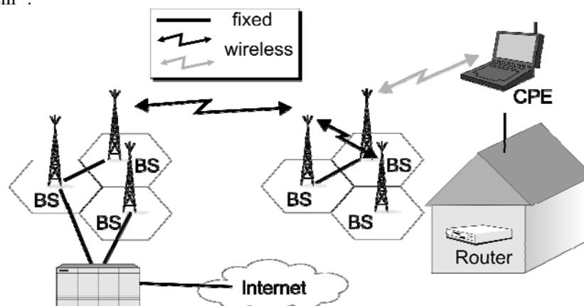
**Figure 6: Wireless Broadband Access Architecture**
