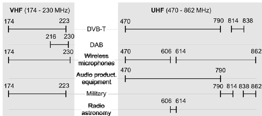
**Figure 4: Spectrum utilization in the VHF and UHF bands in Germany<sup>54</sup>**
